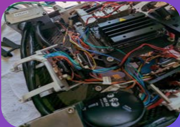
Close-up of Boreas's internals—GPS, ESCs, and aluminum clamps
