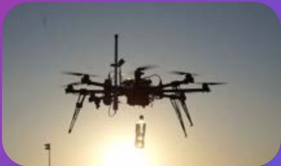
Airdrop Mechanism shown with a water bottle
